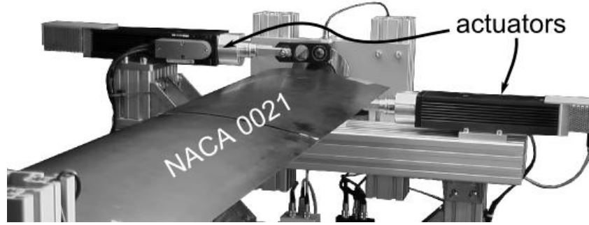
Figure 4. Pair wise arrangement of the linear servo actuators on the side of the light-weight vortex generator airfoil.
