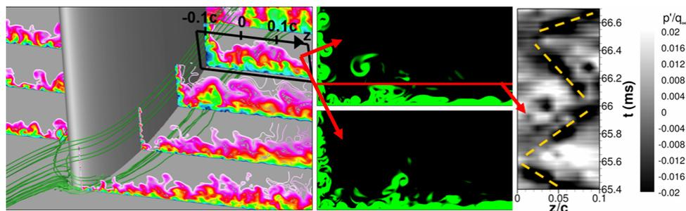
Figure 3: Identification of transverse oscillations of the horseshoe vortex in the convection area
