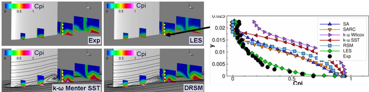
Figure 4: Turbulence modelling effect in the corner area, total pressure losses are displayed
