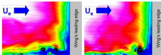
Figure 2: Evidence of the bimodal behaviour of the horseshoe vortex in the symmetry plane (negative axial velocity in blue)
