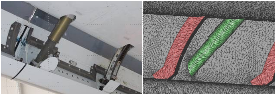
Figure 2: Real and discretized geometry of the slat tracks and the de-icing pipe.
