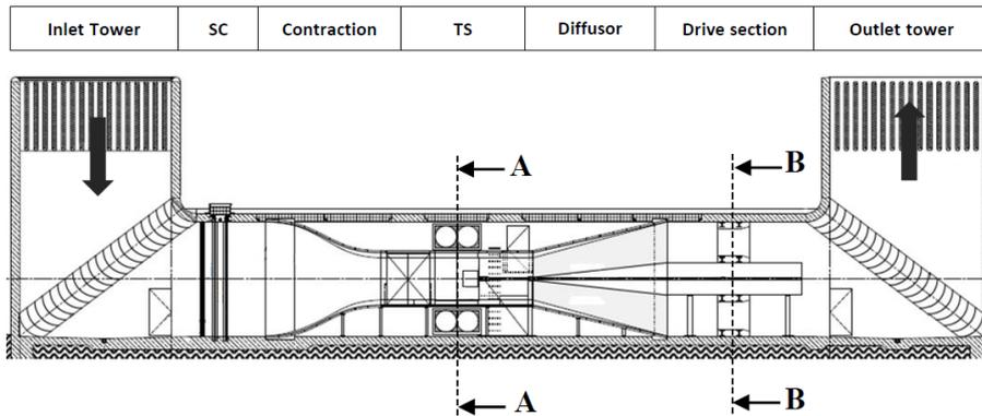
Figure 1: Fan-Test-Facility layout
