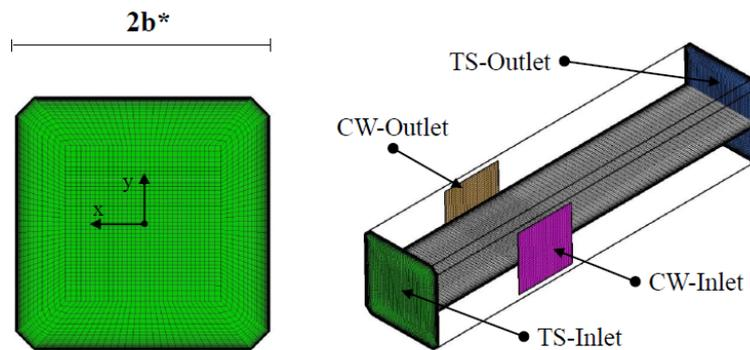
Figure 4: Structured mesh of the test section
