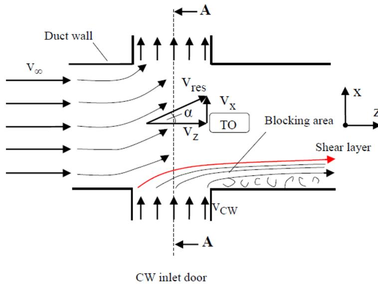
Figure 3: Generating of angles of attack by flow interaction
