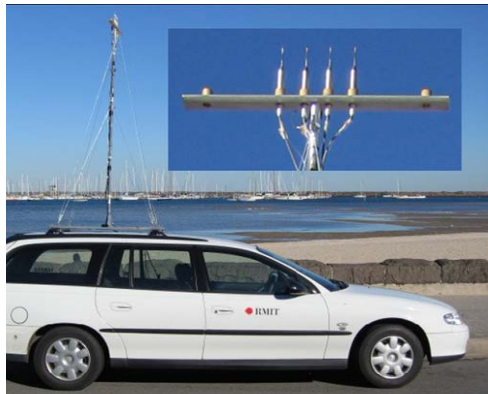
Figure 9 Test vehicle with probe system (inset) and schematic of single head (above)
