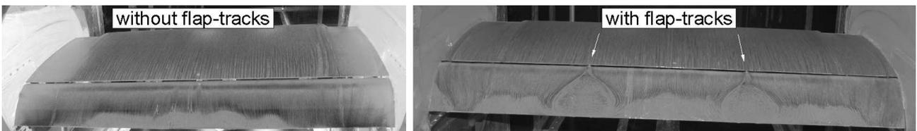
Figure 15: Oil flow visualisation of flap-track influence with step-nose configuration at  $\alpha = 4^\circ$
