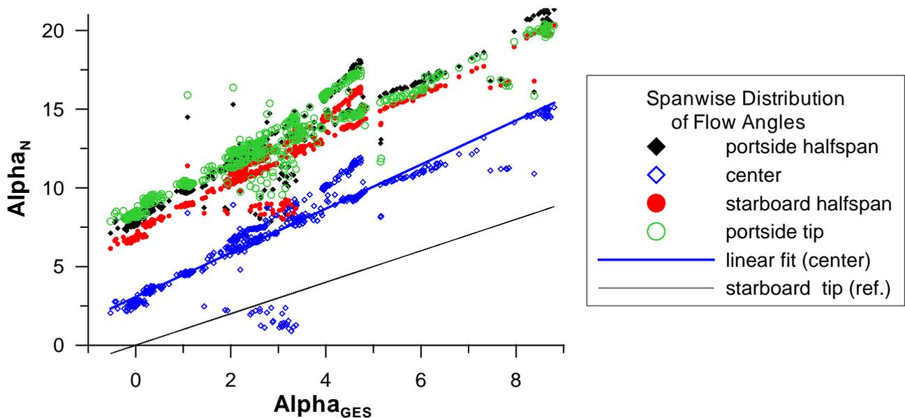
Figure 8: Local flow angles at probe positions 1..4 drawn vs. Flow angle at global probe position
