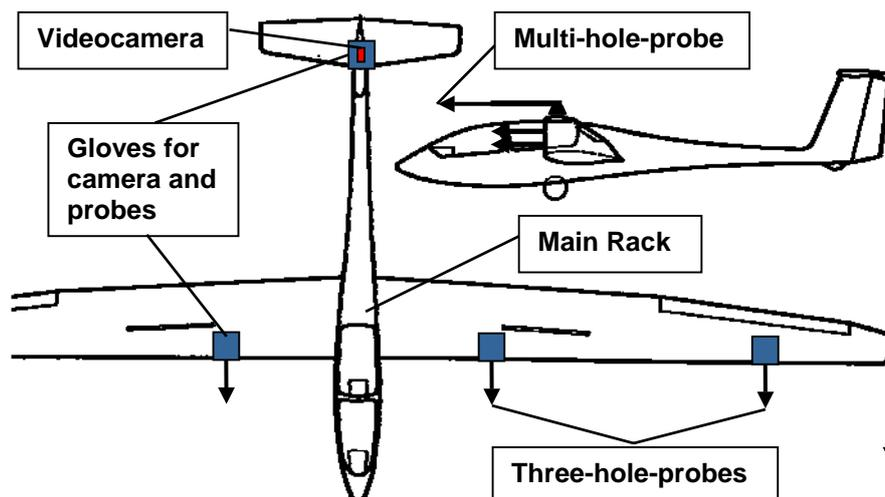
Figure 4: Intended setup on the Twin Astir for thermal flight measurement
