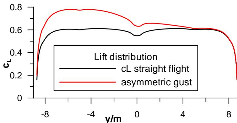
Figure 9: Change in lift distribution caused by an asymmetricly hitting vertical gust. Total lift increases due to average upwind. Induced drag increases only by 1.6%.
