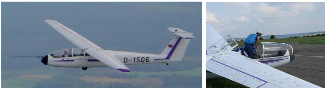
Figure 3a,b: L-23 Super Blanik with 4-hole-probe on a noseboom and camera on tail observing flow structures on the wing
