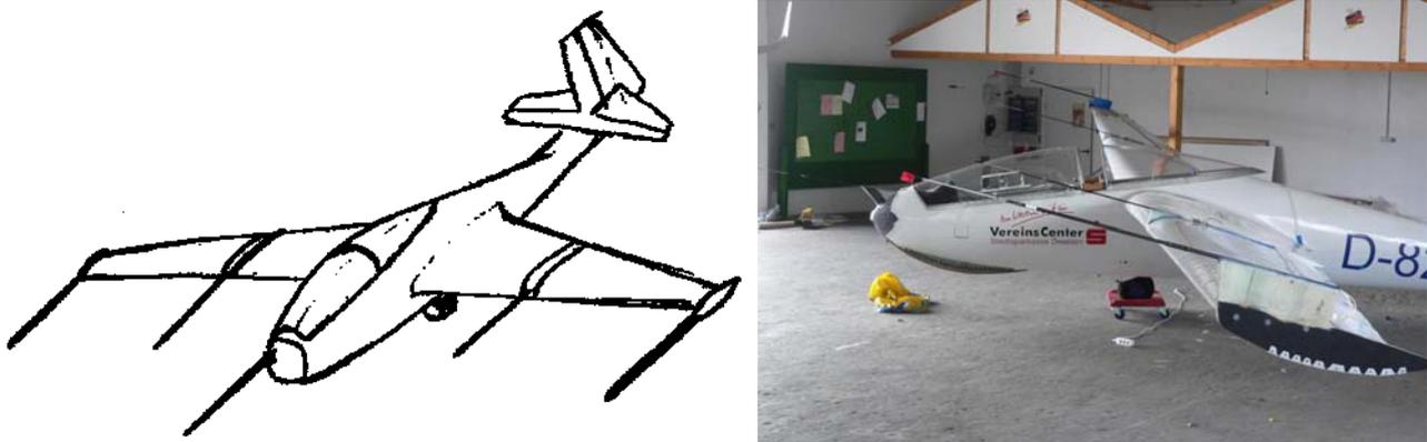
Figure 3a,b: Scetch and photograph of the SZD-9 Bocian equipped with flow angle probes for thermal flight investigation
