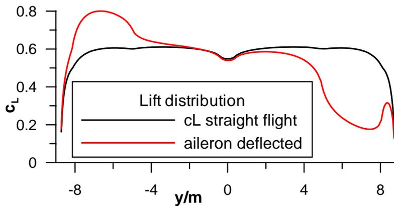
Figure 2: Change in lift distribution caused by aileron deflection with lifting line. Due to differential deflection ( $+5^\circ, -10^\circ$ ), total lift is slightly decreased. Induced drag increases by 22%.
