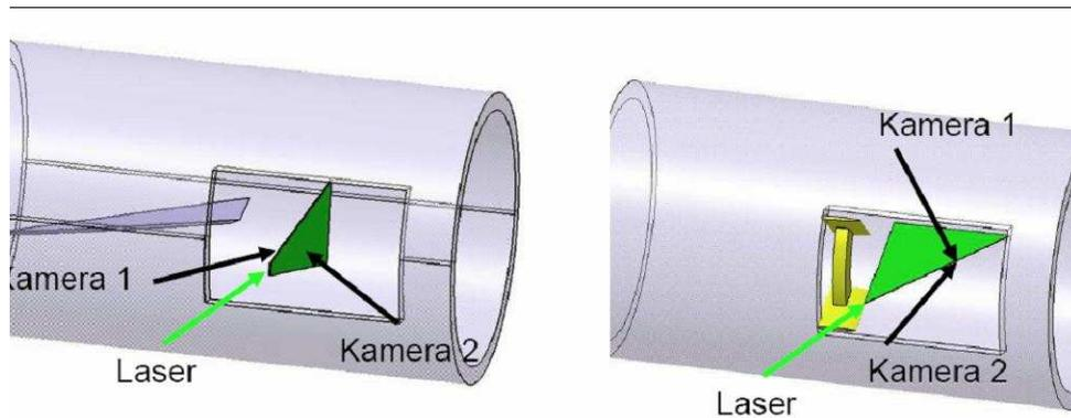
Figure 14: Sketch of the PIV setup showing the laser sheet
