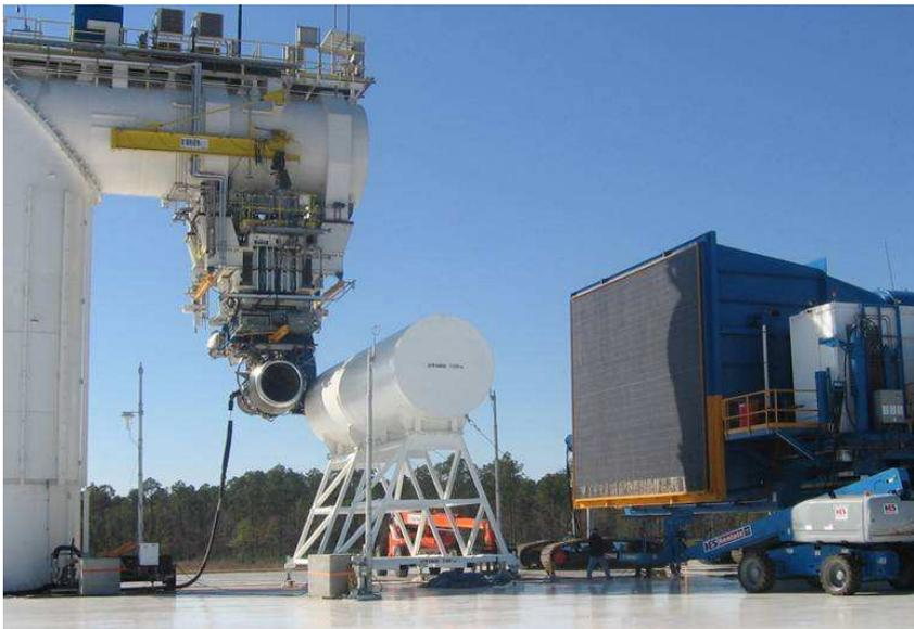
Figure 3: Engine test in crosswind at Rolls-Royce Stennis test facility
