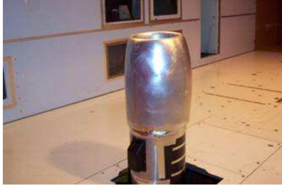
Figure 2: Model scale intake test in crosswind without fan in the ONERA F1 wind tunnel at full scale Reynolds numbers
