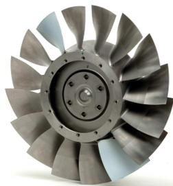
Figure 6: Titanium blisk Rotor 1
