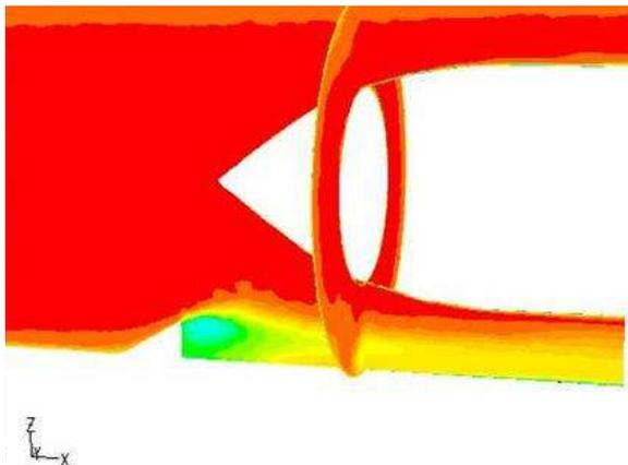
Figure 9: Total pressure simulated by CFD of a backward facing step type distortion generator implemented in the TU Darmstadt compressor rig
