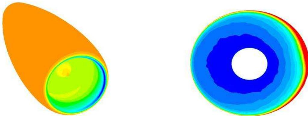
Figure 1: Disturbed flow in an isolated engine intake under crosswind from right (left figure: static pressure, right figure: total pressure loss at the fan face)
