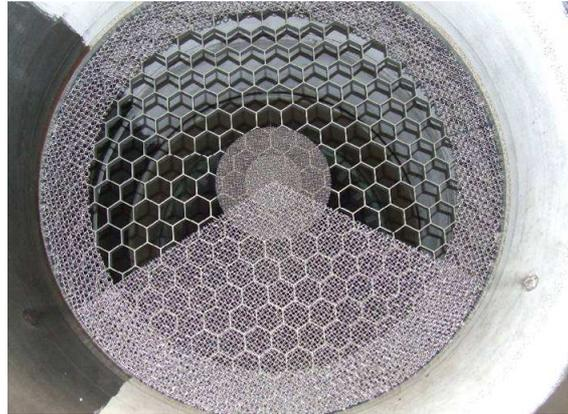
Figure 8: Distortion screens used to provide total pressure loss patterns in terms of CDI and RDI
