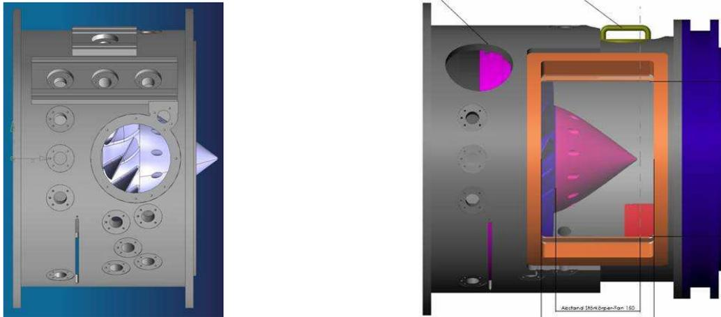
Figure 13: Original rotor casing (left) and new design (right) with PIV access (window made out of quartz)
