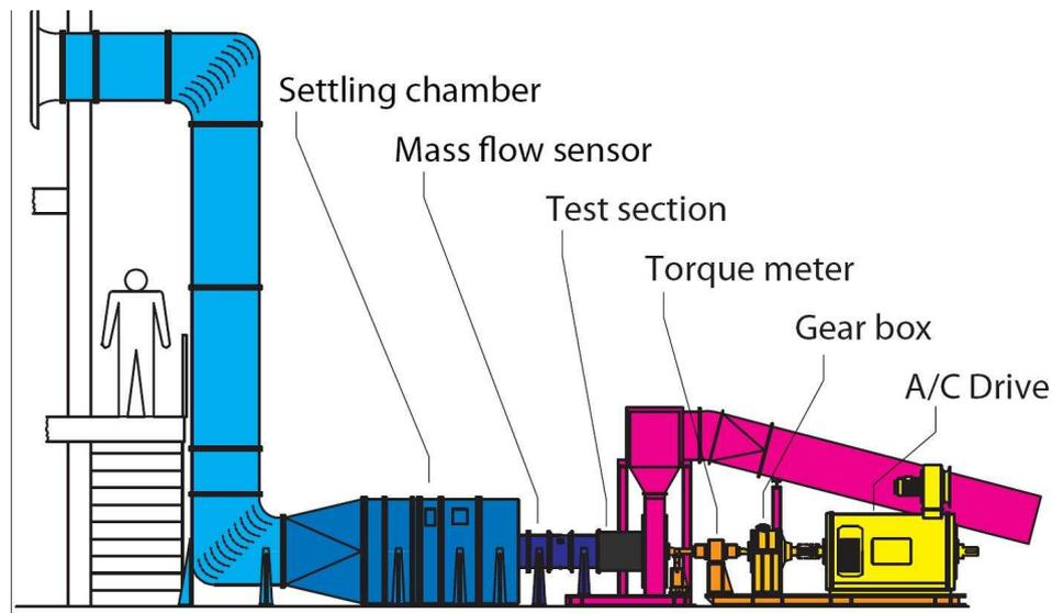
Figure 4: Transonic compressor rig at the TU Darmstadt
