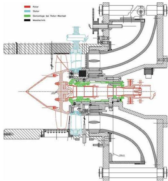
Figure 5: Details in a vertical cut of the compressor
