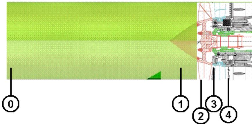
Figure 12: Schematic view of the TUD compressor rig showing new parts and measurement sections
