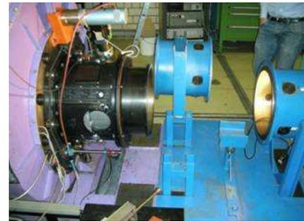
Figure 7: Removable onflow section into the compressor
