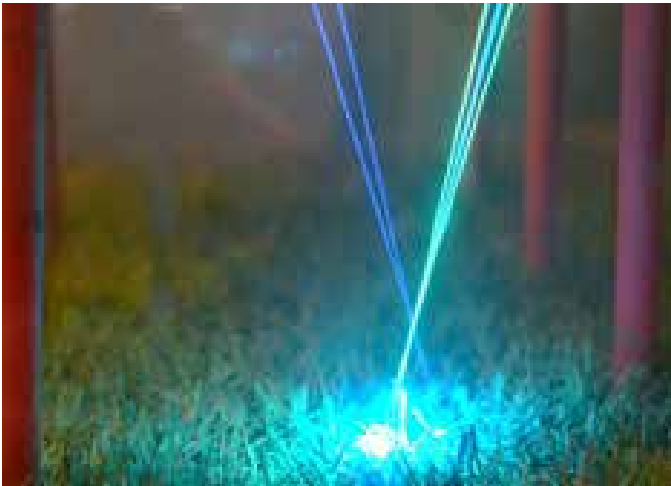
Near bed velocity measurements with a 3D-Laser-DopplerAnemometer in a flume study on flow-vegetation interaction Source: J. Aliaga-Villagrán (LWI)
