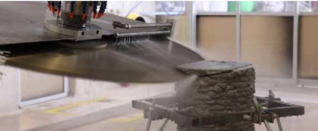
Recycle: Cutting of dry joint for reversible connections, applicable for salvaged as well as for newly printed structural elements
