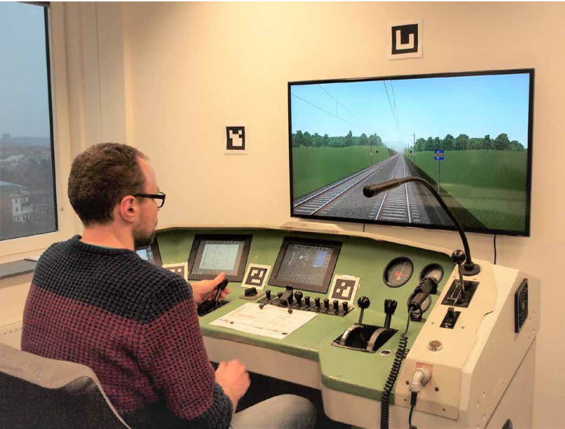
This Side: Train driving simulator in the Virtual Railway Operations Laboratory (Picture: Pachl)
