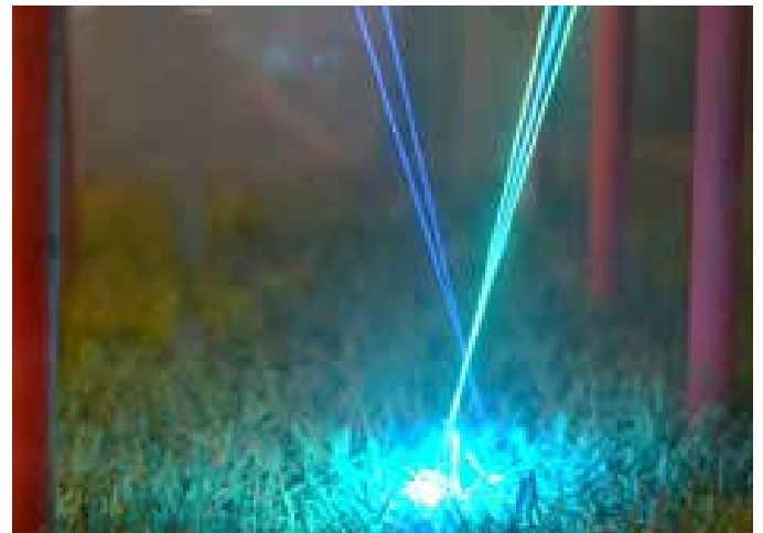
Near bed velocity measurements with a 3D-Laser-Doppler Anemometer in a flume study on flow-vegetation interaction Source: J. Aliaga-Villagrán (LWI)
