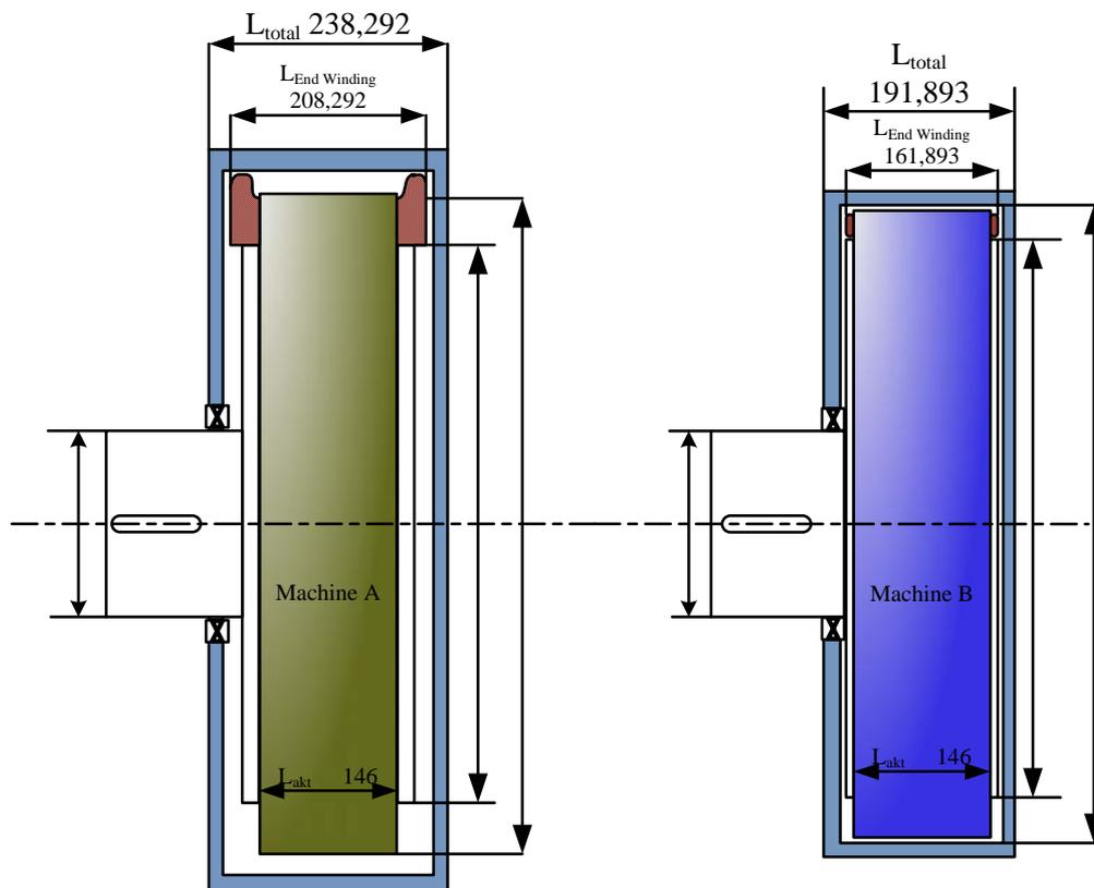
**Figure 4:** Dimensions in mm of Machine A and B for  $P_{mech} = 79,23$  kW and speed =  $300 \text{ min}^{-1}$
