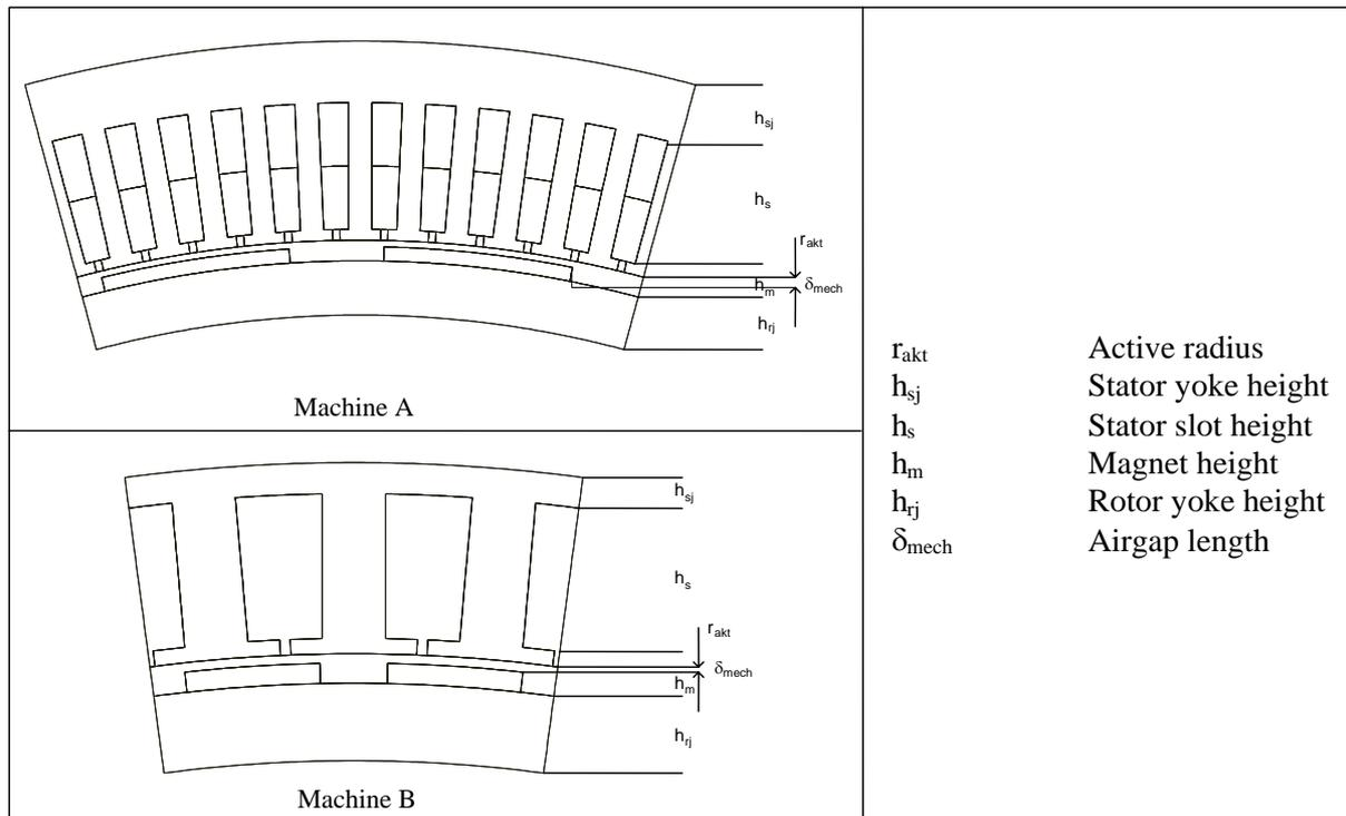
**Figure 1:** Geometry of PMSM
