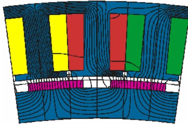
**Figure 3:** Flux lines for Machine B
