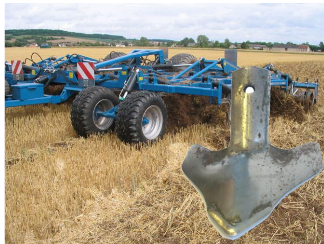
Figure 1: Typical wearing on a cultivator tine [source: Köckerling / Wearpoints]
